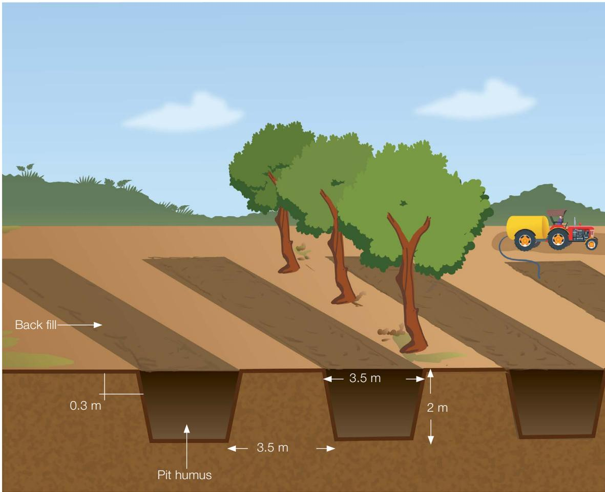
Figure 3: Typical Plan of a Trenching Site
