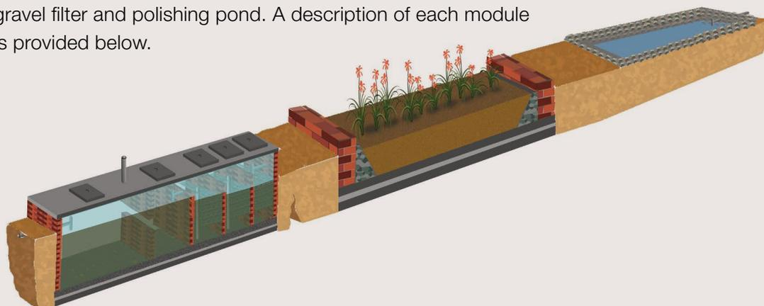
**Integrated settler and aerobic filter**
